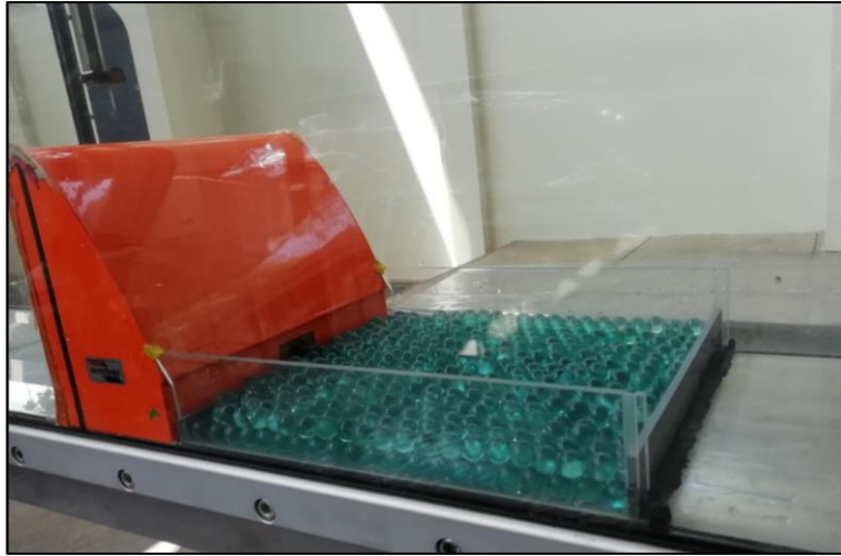
Figura 21: Disipador Gravel Box Stop Logs: D (original)
